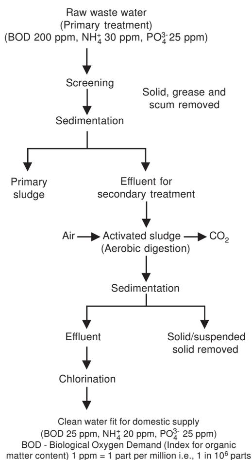
Fig. 7. Municipal waste water treatment (Primary and Secondary)
