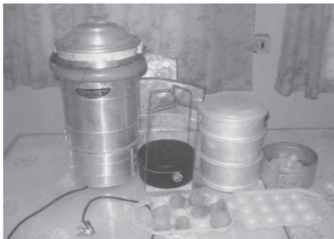
**Fig. 4.** (From left) Electrically operated closed circuit smokeless oven. Nozzleless kettle contains 6 cups of tea. Food container arranged vertically in this oven. Oven containing paper pulp balls. In front paper pulp balls in the plastic dice (use for carrying eggs)
